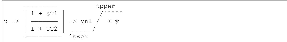
Exports four variables: state  $x$ , output before hard limiter  $ynl$ , output  $y$ , and AntiWindup  $lim$ .
