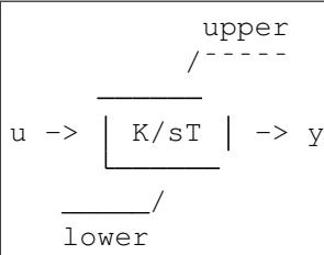
Exports a differential variable *y* and an AntiWindup *lim*. The initial output must be specified through *y0*.
