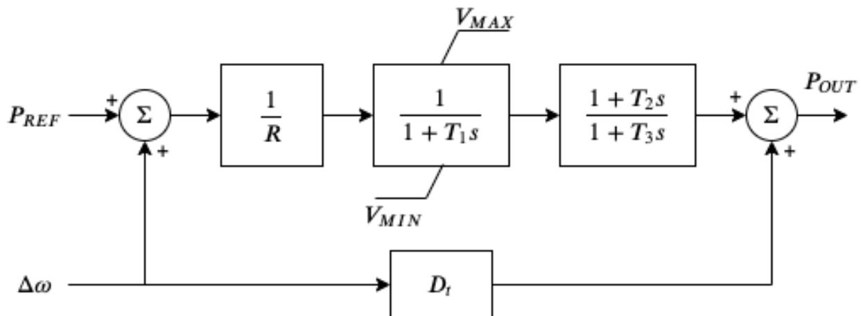
This model is composed of a lead-lag transfer function and a first-order lag transfer function with an anti-windup limiter, which are sufficiently complex for demonstration. The corresponding differential equations
